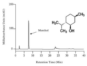
Figure 2 HPLC chromatogram of menthol isolated from M. longifolia leaf oil.
