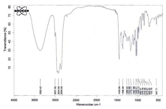
Figure I FTIR spectrum of menthol isolated from M. longifolia leaf oil.
